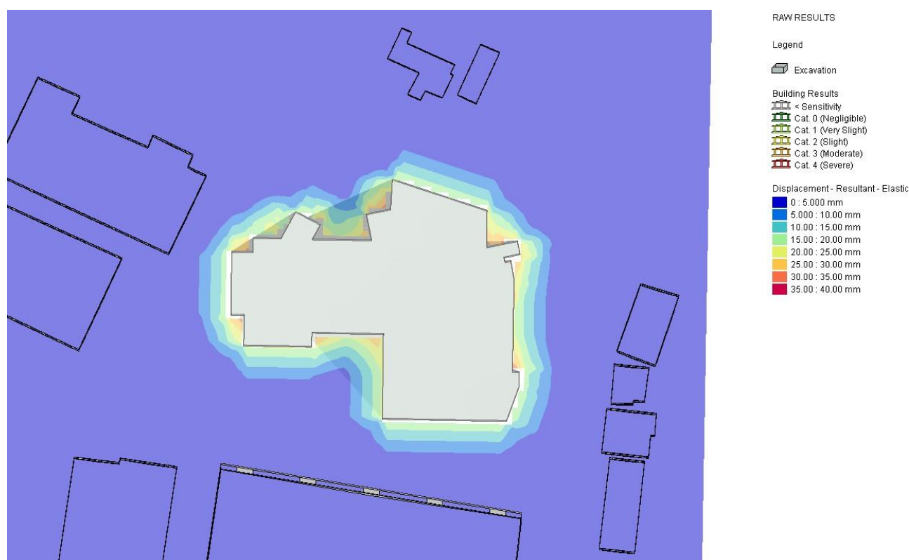
Figure 5.2: Plan of XDisp output of ground movement due to basement excavation
